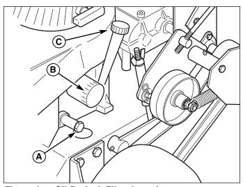
Figure 3. Oil Drain & Filter Locations
